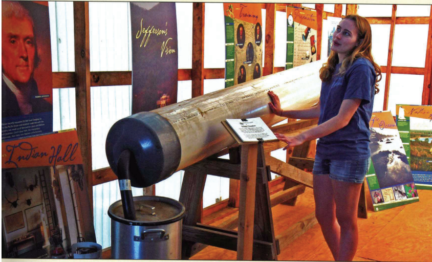
Summer intern Jennifer Bell explains the contraption used to steam ship frames and planks so they would bend. She also demonstrates knot tying for a group of visitors.
